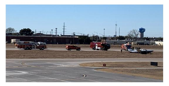
On Saturday, January 29, the left main gear of a Cessna 421C failed and detached when it landed at Addison Airport. The plane slid off the runway and Addison Fire Department was dispatched to respond to the incident. The pilot and four passengers who were on board were not injured. The runway was closed for several hours until an aircraft retrieval specialist was able to remove the small plane.
