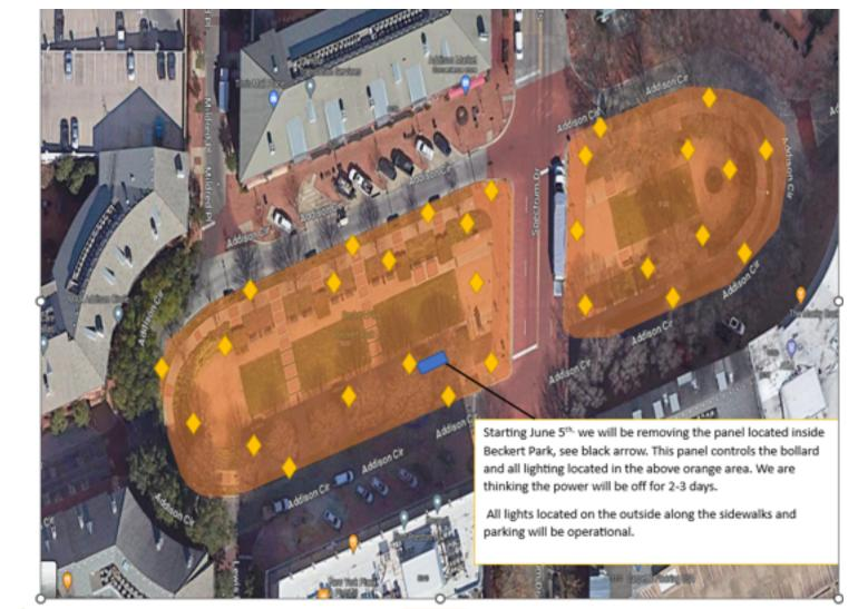
Light poles without power. Panel being replaced. 24 bollards in these marked areas will be replaced.
