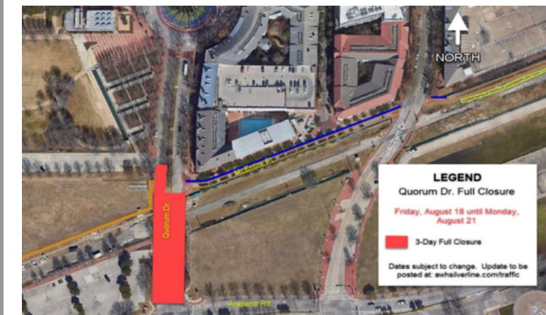
9am until Monday, August 21 at 3:30pm. The closure is needed to demolish the temporary railroad crossing and install ballast, track ties, and rail. Crews will reopen the lanes as soon as the work is completed. Detour signs will be posted, but drivers are encouraged to consider alternate routes while this work is taking place.
