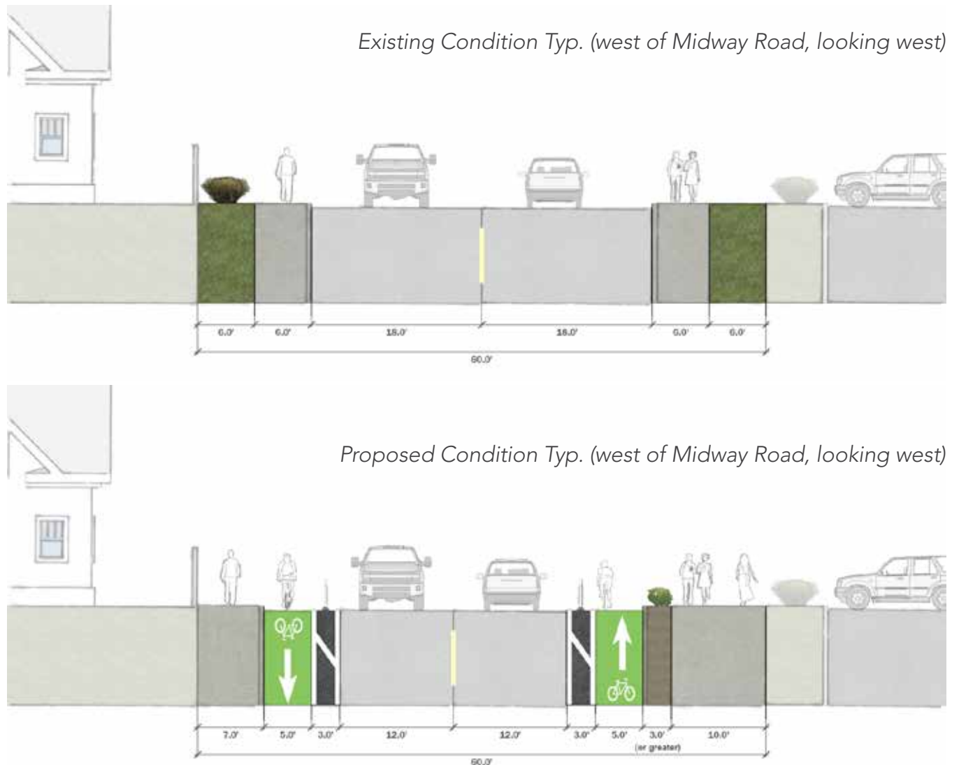
Figure 5-2: Beltway Drive Bike Lanes and Wide Sidewalk
