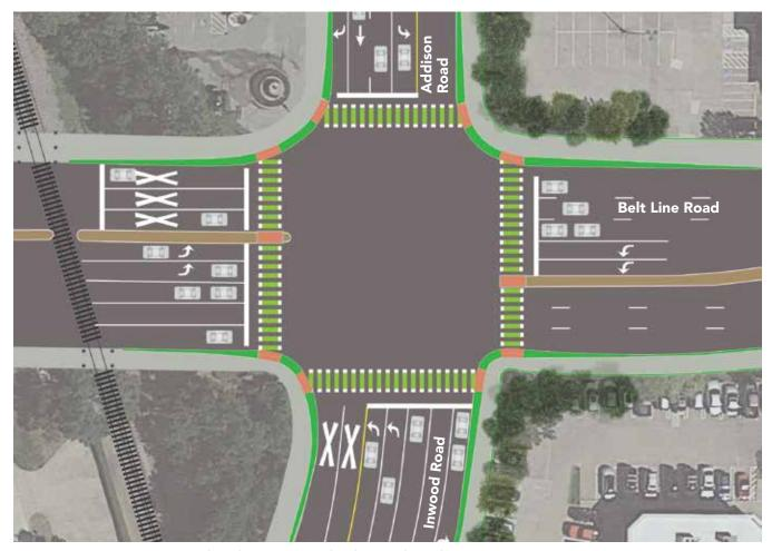
Figure 4-12: Prototypical Belt Line Road Bike and Pedestrian Crossing
