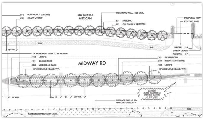
Figure 5-5: Midway Road Construction Drawings
